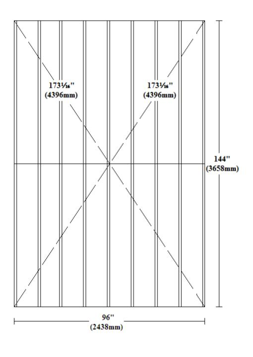
NB:- Floor joists run from gable to gable.
